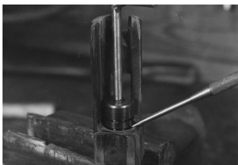
Chamber Gauge verifies that the chamber in this 12 gauge auto barrel is 2¾", as gauge seats to the forward, (or 2¾") ring in the gauge. Note the Chamber Gauge Handle on gauge.
