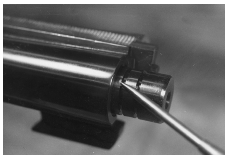
Classic example of short chamber. After thorough cleaning, chamber will not accept gauge to full 2¾" depth. This particular chamber measured 2½" prior to rechambering.
