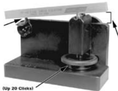
Sear on Power Fixture ready to stone secondary angle
