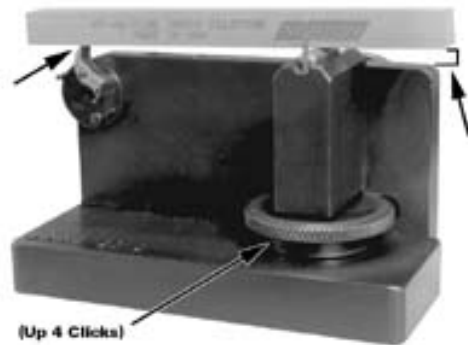
Sear on Power Fixture ready to stone primary angle
