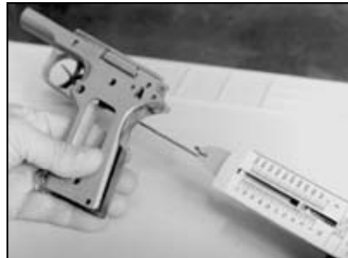
Combined sear and disconnector pull weight shows 16 oz.
